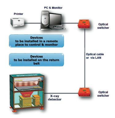
The above devices can be connected together via optical cable or via customer's LAN system. A typical connection is as sown in the figure above.
