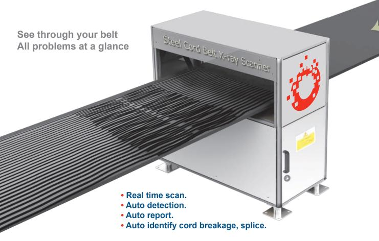
Steel cord conveyor belt X-ray inspection system (coal mine explosion-proof grade) uses X-ray to scan entire conveyor belt in a timely and accurate manner (up to 0.8 mm resolution) and submit the images to a dedicated software which is able to conduct intelligent, holistic inspection on a up damages such as broken cords, rusted/corroded cords, kinked cords, missing cords, splices, etc. conveyor belt and provide diagnostic data.
